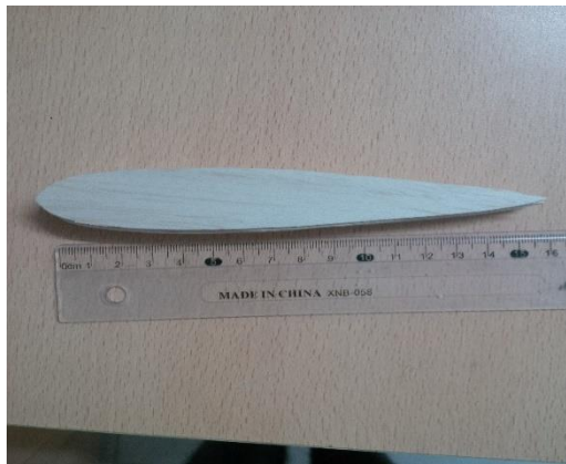
Figure 4.1: Ribs from balsa wood
