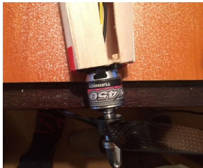
Figure 4.13: Mounting of motor
