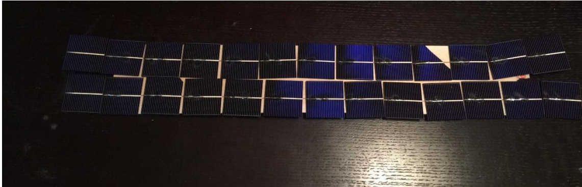
Figure 4.17: Solar cells in series and parallel
