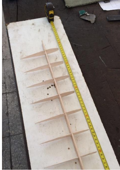
Figure 4.3: Spacing of ribs
