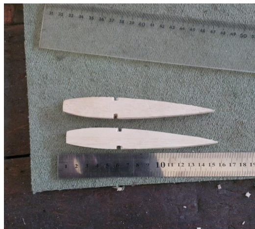
Figure 4.2: Cut ribs for placing spar
